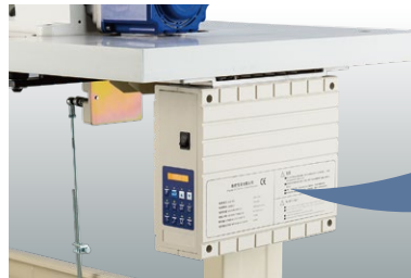
Control box and the operation panel
